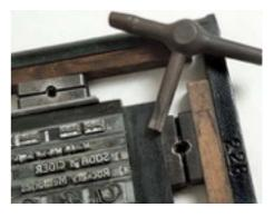
When satisfied, the whole together with any "blocks" of stock pictures, the school crest etc, was assembled into a heavy cast-iron frame, the "Chase", spaces filled with wooden "furniture" and securely locked up with clamps - "Quoins" to create the finished page layout, the "Forme" ready for transfer to the printing press.
