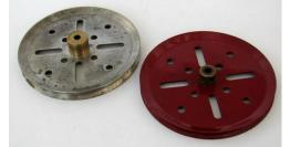
3) Pulley 1" diameter with boss, part no. 22. The standard 3/8" boss was introduced in 1913 (in place of keyways), but had only one tapped screw hole until March 1927 (this applies to all types of wheel and gears). Afterwards two tapped holes were provided, so this is a useful means of dating these items.
