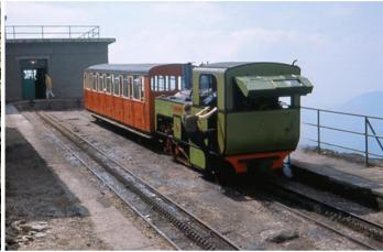
The tramway is of 800 mm gauge, built on Swiss mountain railway principles, and runs seven engines of which three are 1895 originals and the rest built to a modified design in 1922. Operation is on the Abt rack system, with each engine pushing one carriage up to the summit via three intermediate crossing loops. The maximum gradient is 1 in 5, and a speed limit of 5 mph in both up and down directions gives a
