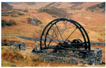
It was formerly connected by horizontal square-section wooden pump rods to the shaft headgear some distance off, which retains the pump mechanism. The equipment was installed circa 1870 and the mine was working until about 1893. This picture shows the wheel in the background at right, and the headgear towards lower left, fenced off for safety reasons......
